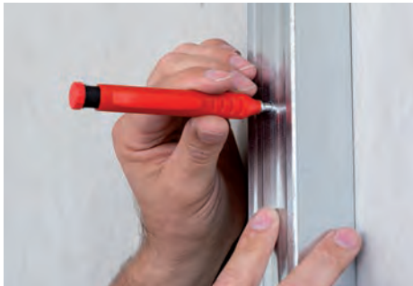
TLM2 for markings up 1.7 inches depth.
