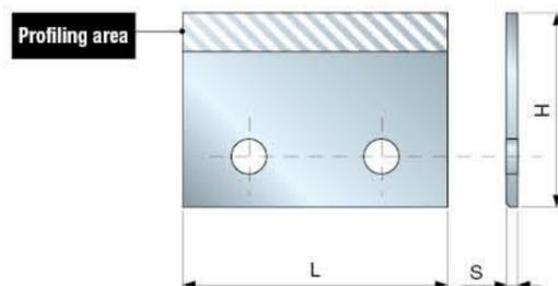
Profiled knives with 2 mm thickness.
