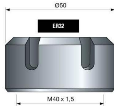
Locking rings suitable for universal high precision chucks with MP06M collet.
