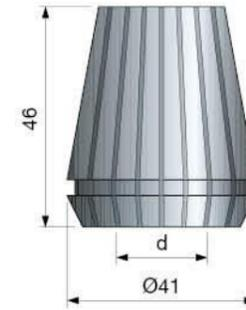
Collets for router bits with cylindrical shank. Suitable for MP08MDC AA9 and MP10MDC AA9 chucks.
