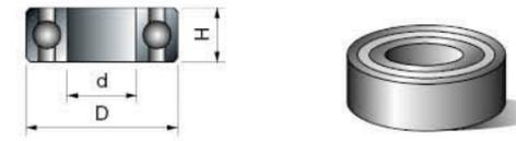
Ball bearing for router bits.
