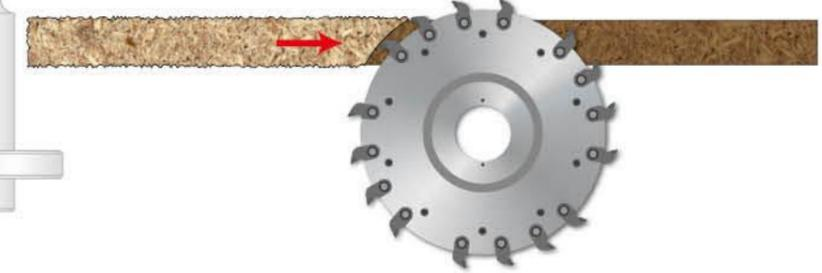
These tools can be stacked and used in multiples thus enabling the machining of a wider area.
