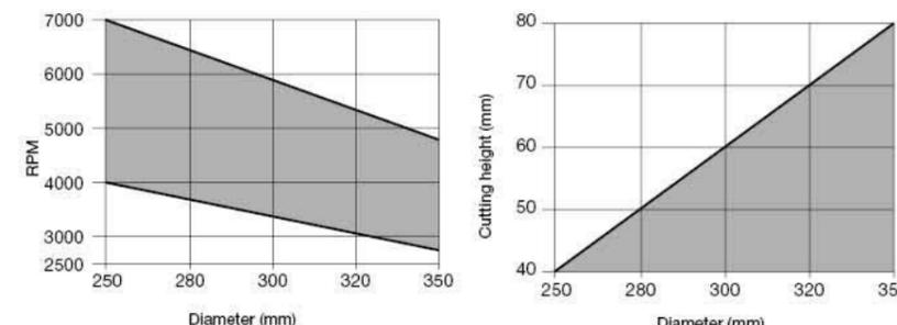
Minimum and maximum RPM based on the blade diameter.
