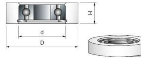
Cylindrical rub collars for ball bearing.
