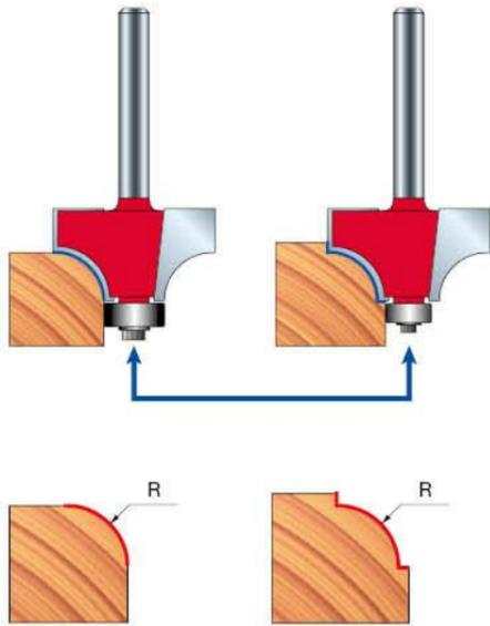
By ordering a smaller ball bearing and step washer you will be able to obtain a different profile:
