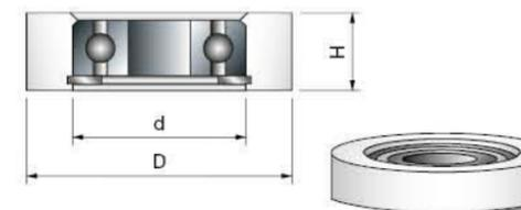
Cylindrical rub collars for ball bearing.
