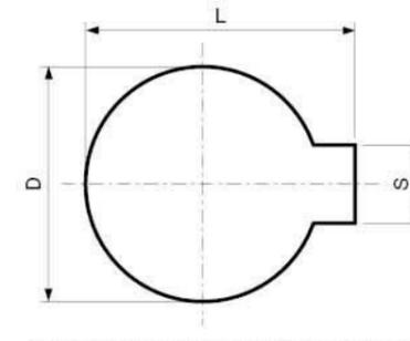
Standard keyway for existing cutterheads.
