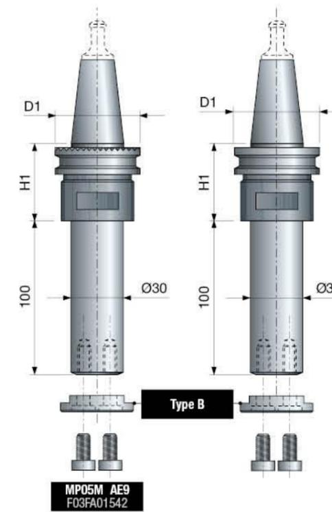
Spindles for overhead CNC machines with ISO30 shank for Ø30 mm tools bore.
