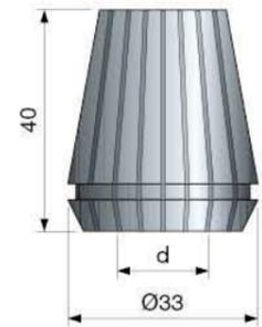
Collet for router bits with cylindrical shank. Suitable for MP06MD, MP08MDC AA9 and MP10MDC AA9 chucks.
