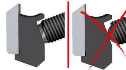
Proper locking is obtained when the flat surface of the spherical insert completely adheres to the wedge.
