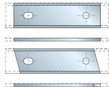
Disposable knives with 2 cutting edges without side clearance.
