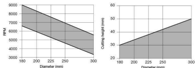
Minimum and maximum RPM based on the blade diameter.
