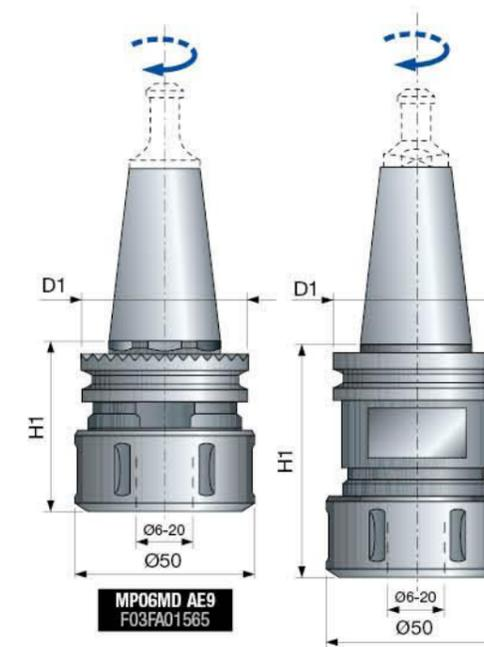
Chucks for overhead CNC machines with ISO30 shank.
