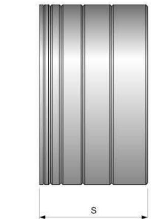
Standard spacers sets suitable for cutterheads.
