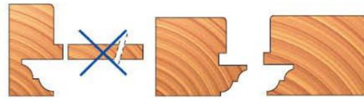
Jamb and transom with ST12MG-801 set: by cutting the tenon as shown, the counter profile with anti-torsion pin is obtained.
