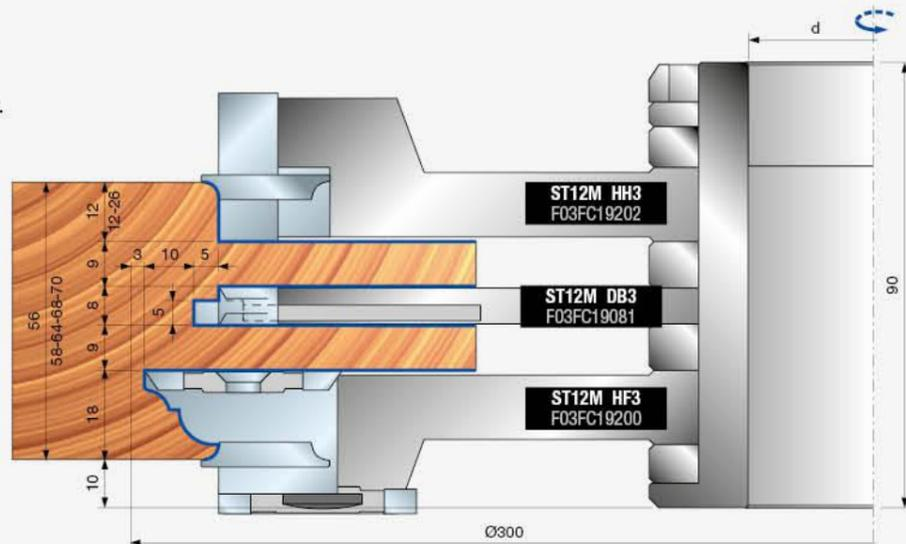
Scribes with 3 mm external rounding for cutterheads: ST12M HG3 - ST12M HF3
