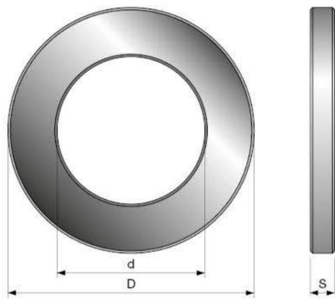
Special spacers suitable for cutterheads; minimum thickness 1mm.
