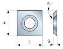
Wide range of squared spurs with 4 cutting sides with variable Carbide types and relief angle to cover all available materials.
