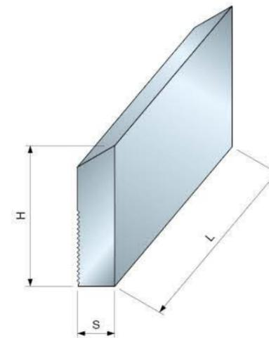
Profiling HSS knives with serrated surface.
