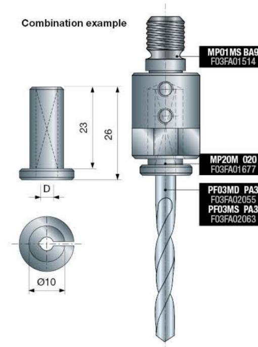
Adaptors for drill bits (as PF03MD/S) suitable for MP01MD/S chucks.
