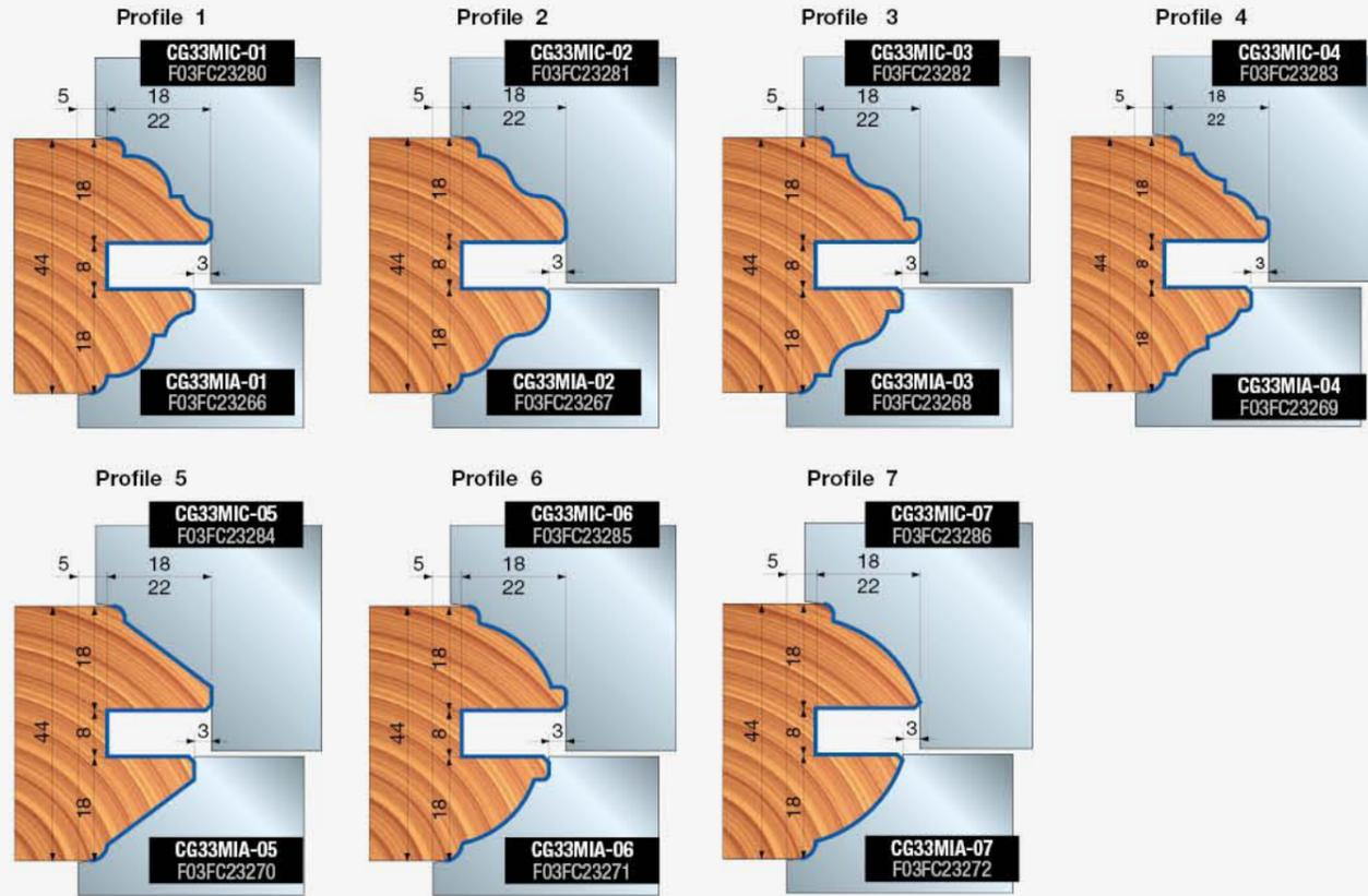
Profiling without external rounding - Knives for cutterheads ST16MIAC13 - ST16MICC13
