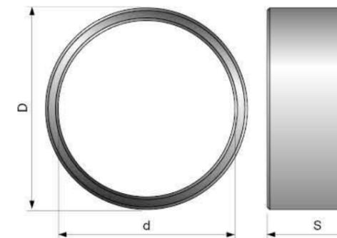
Standard reduction rings suitable for cutterheads.
