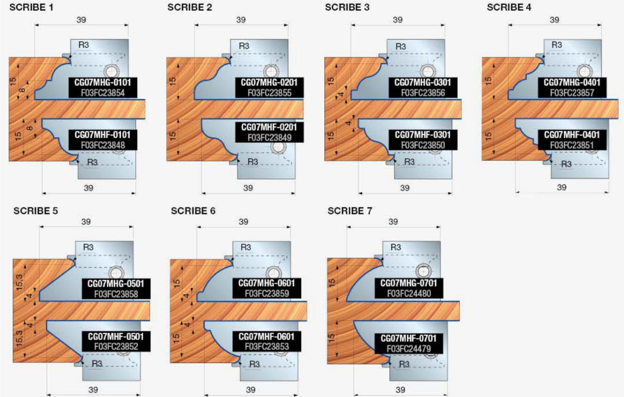
Scribes without external rounding for cutterheads: ST12M HG3 - ST12M HF3
