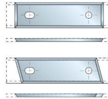
Disposable knives with 2 cutting edges with side clearance.
