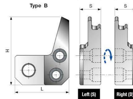
Deflectors suitable for standard IG13M sealing inserts as anti-kickback device.
