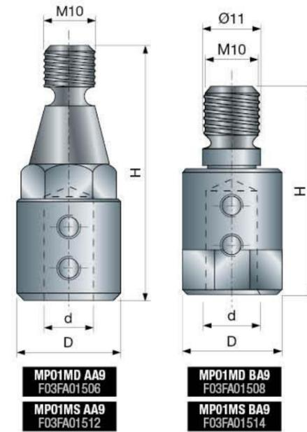
Freud standard chucks for router bits.
