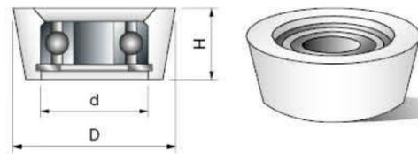
Conical rub collars for ball bearing.
