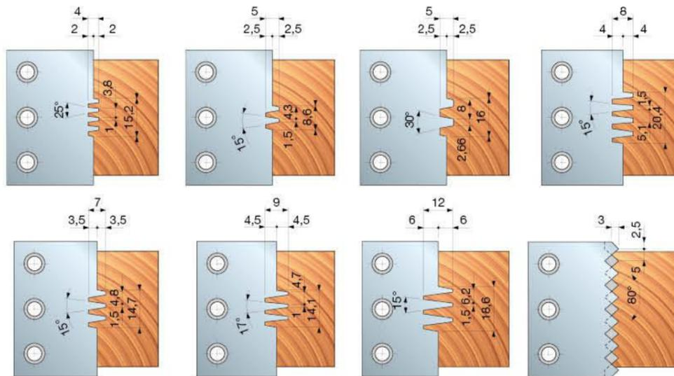
PCN130 is suitable for jointing too, with 8 different joint proposals with adjusting system to manage regular, tight and loose joint.
