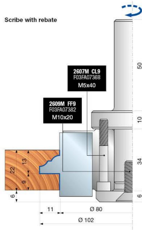
To obtain a 5 mm tenon, it is necessary to use a washer ST07M-109 (1 mm thick) under the SR06MDAH302 (7 mm thick) inserts. The washer must be ordered separately.
