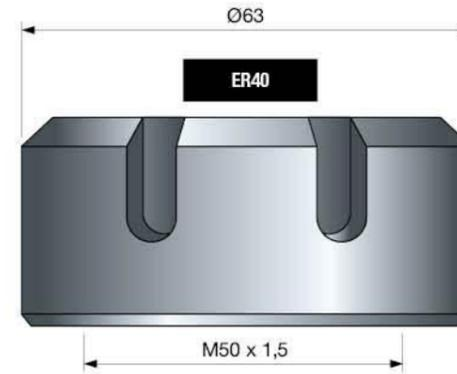
Locking rings suitable for universal high precision chucks with MP16M collet.
