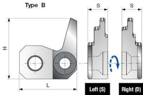
Deflectors suitable for standard IG10M sealing inserts as anti-kickback device.
