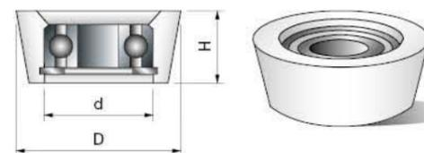
Conical rub collars for ball bearing.
