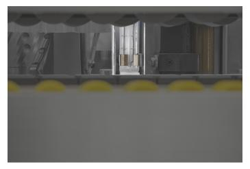
**Lighting of the machine interior**The high efficiency LED lamp improves the view of the operating units inside the machine without needing to open its door. This device is particularly useful for a safe observation of the machine during the processing.
