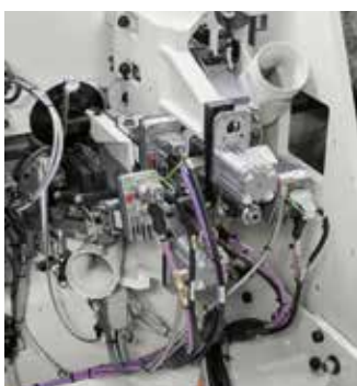
RAS-A edge scraping unit Simple and quick change of the machining radius.
