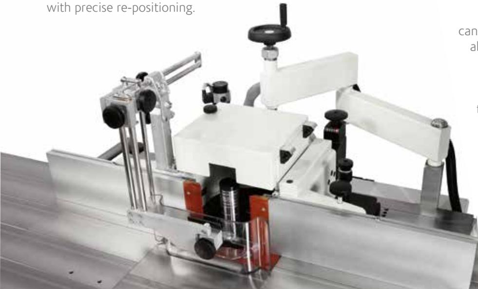
machining with tools on the spindle head carried out with the "Flex" fence
