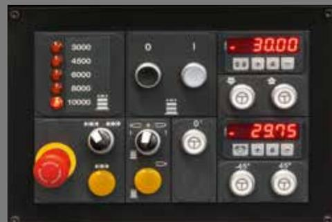
Powered operating unit movement with digital readouts.
