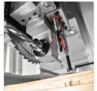
BRC-S operating unit for grooving, routing and drilling both vertically and horizontally.
