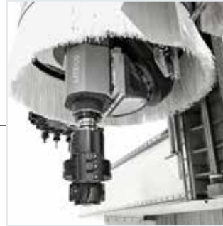
KPX 5-axis operating unit with 17kW electrospindle.
