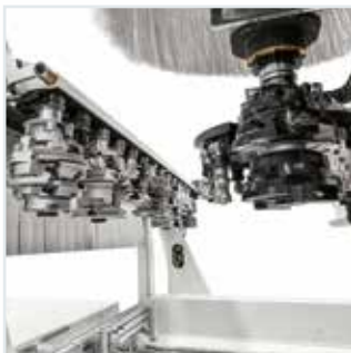
FAST 16 on-board linear tool changer located on board the mobile gantry to optimize tool changes. A dedicated pick-up for large diameter saw-blades is available.
