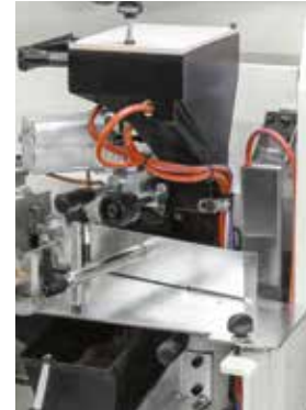
SGP-E glue pot Perfect joint line and use of EVA and PUR glue.
