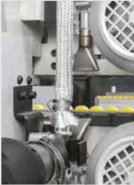
ID 3000 edge brightening unit It brightens the colour of plastic edges by heating them with hot air.
