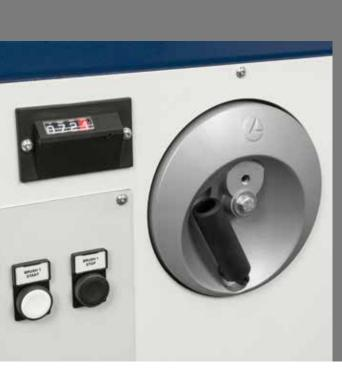
**Operating units lifting** by means of handwheels and numerical readout.
