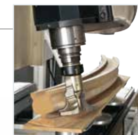
PRISMA machining head with 5 axes electrospindle.
