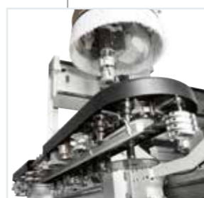
Chain tool store with 48 positions anchored to the mobile gantry structure, developed for managing heavy and large tools.
