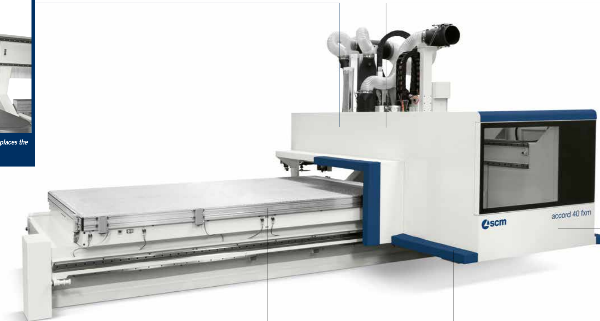
Bars worktable configurable with clamps and suction cups, ideal for the processing of solid wood.
