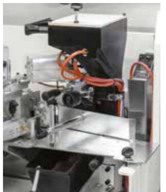
SGP-E glue pot Perfect joint line and use of EVA and PUR glue.
