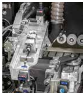
RAS-R edge scraping unit Simple and quick changeover between 2 radii.
