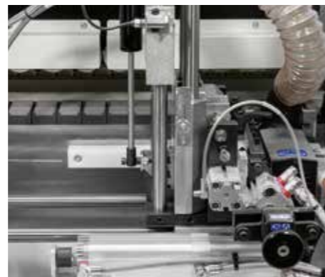
Round 1-V unit Rounding of straight or shaped corners of up to 60mm thick panels; separate machining of front and rear corners. Possibility of machining separate front and rear corners. Motor changeover for processing the second radius.
