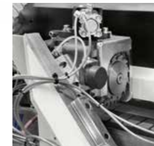
K-2 Radius end cutting unit Cut and radius in a single operation.
