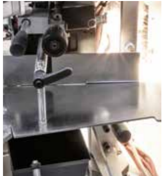
Preheating lamp For excellent edgebanding even at low room temperature.
