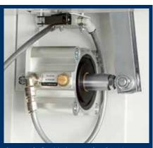
**Automatic feed belt centering** for a longer lifespan of the belt.
