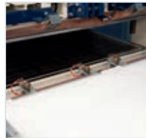
The bottom mobile platen is milled to realize all the circuits that allow creating vacuum.
