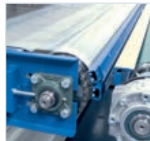
Mylar tensioning device , simple and fast replacement.
