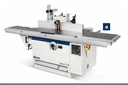
The "PRO-10" tenoning table can be retracted easily and within a few seconds to leave the machine ready for profiling (**a**) or moulding (**b**) operations.
