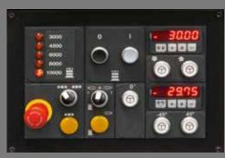
**Powered operating unit movement with digital readouts.** Maximum precision and ease-of-use. The "eye-S" control can manage the inverter for the adjustment of spindle rotation speed. (option)
