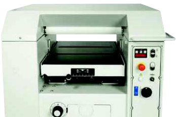
thickening table with two removable idle rollers It assists the feed for demanding pieces.
