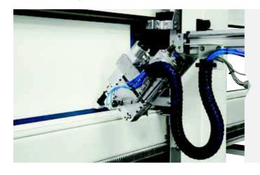
5-axis automatic stapler for the rear side of cabinets, to be installed on the action tf clamp. Ideal solution for producers of kitchen, bedroom and bathroom furniture.
